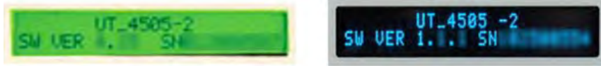
(LEFT) Liquid Crystal Display (LCD) – Initially Released Chassis (RIGHT) Vacuum Fluorescent Display (VFD) – Current Production Unit
