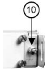
Figure 4-12. Unit Ground Connection
